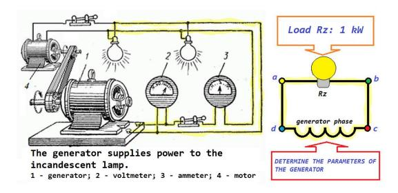
First, we need the generator parameters. We will calculate the generator according to the classical scheme of a frame rotating in a magnetic field between two poles.
