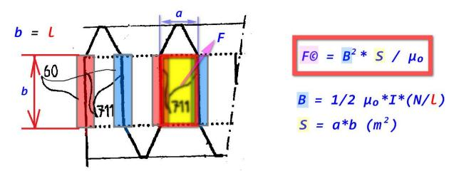
The electromagnetic moment with the sum of the Ampere forces and the electromagnetic traction force, will preliminarily have a value: M = (0.78 + 0.157 = 0.937) \* (0.35 / 2) = 0.163 N \* m, which will be, in the need for the drive power of the generator motor, taking into account the coefficient 1.2 at idle:
