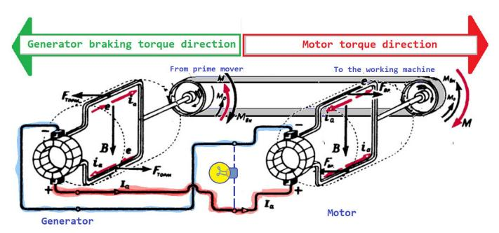
In the picture I have depicted a DC motor housing and a DC generator housing connected by a belt drive to each other. The frames of the electrical conductor are closed with each other through the collector brush. We assume that we will also have a payload.
